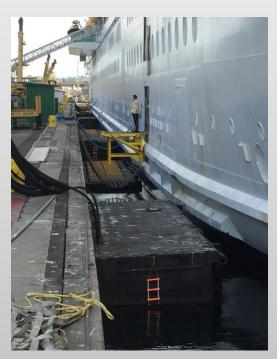
Standoff (or Camel) Barges serve to hold the Cruise Ship off the pier for servicing in port
